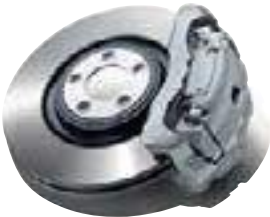
355MM FRONT AND 325MM REAR BRAKES
