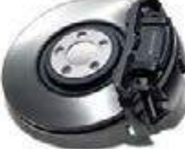
380MM FRONT AND 325MM REAR BRAKES
