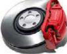
380MM FRONT AND 376MM REAR BRAKES
